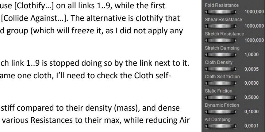
When running the sim, I found out it did not work. The first clothified link did stick to the collision object link left to it but the chain broke at the next link. This means that the chain is moving too fast for the simulation to handle the collision, and pumping up the Steps-to-Frame settings in the [Simulation Settings...] is actually the only way out. But to what extent? The image
