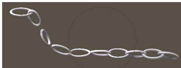
shows the result of Steps set to 128 (the sim takes 10 sec/frame) and further testing reveals that Steps set to 512 (40 sec/frame calculation time) only improves the result a little bit.
