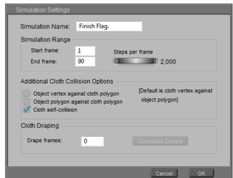
Now I have to fetch the flag to the pole, in such a way that the top vertices of the flag behave like nailed to the vertices and polys of the pole. The pole is in the collection of Collision objects, so putting the flag vertices in the Constrained Group will do.
