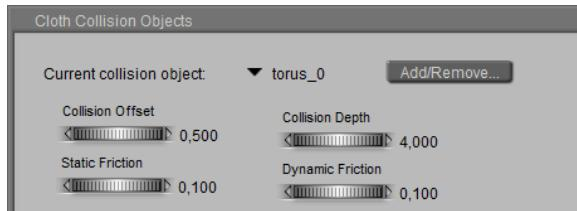
Altering the collision parameters has no effect, as these concern the interaction between the clothified objects and the collision objects only. And the breaking chain shows that the issue is in the interaction between the clothified objects themselves.
