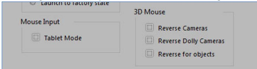
Where I can enable Tablet Mode, that is: a large distance by pen is translated to a small distance in the Document Window, for greater accuracy. And I can alter the behavior of a 3D Mouse, so when I pull it (decrease Z value) the object or camera moves towards me (increasing Z value instead). And so on. This is because other programs might have the positive Z-axis pointing backwards.
