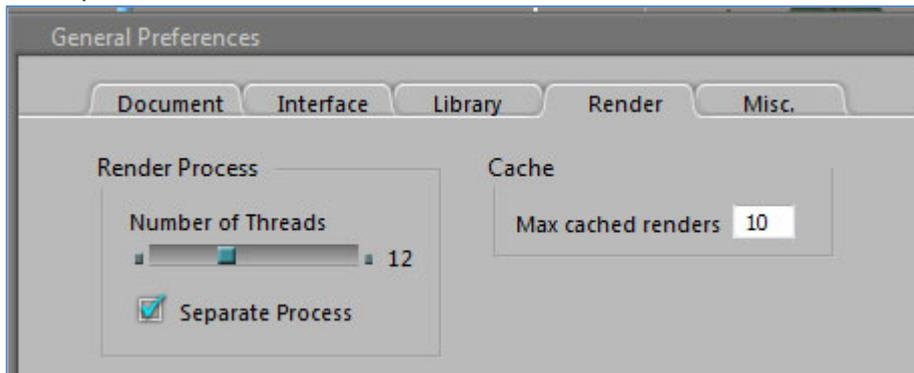
Separate Process (OFF by default) forks out the renderer which therefore is freed from all the hassle from the design process, a memory saver as discussed in the *RAM usage* section. Number of threads should be left to a default (it auto detects the machines maximum). See the *CPU usage* section on how to launch Poser in reduced priority mode, which is a far better mechanism.
